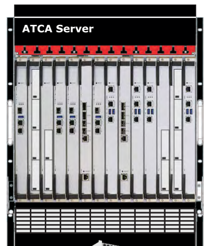
14-Slot ATCA System Full redundancy here in picture with 12 AMC 's
